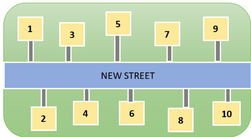
Figure 8 – Numbering along a new street
